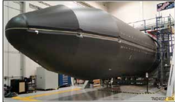
Figure 2.2.5.1-1. Antares 3.9 m Fairing Assembly
